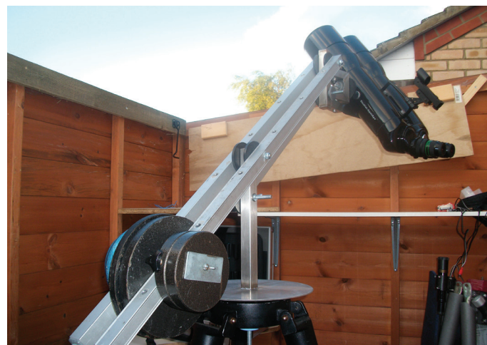
▲ A heavy duty parallelogram mount carrying the seven kilogram 100mm APM binoscope with ease. Image: Mark Radice.
