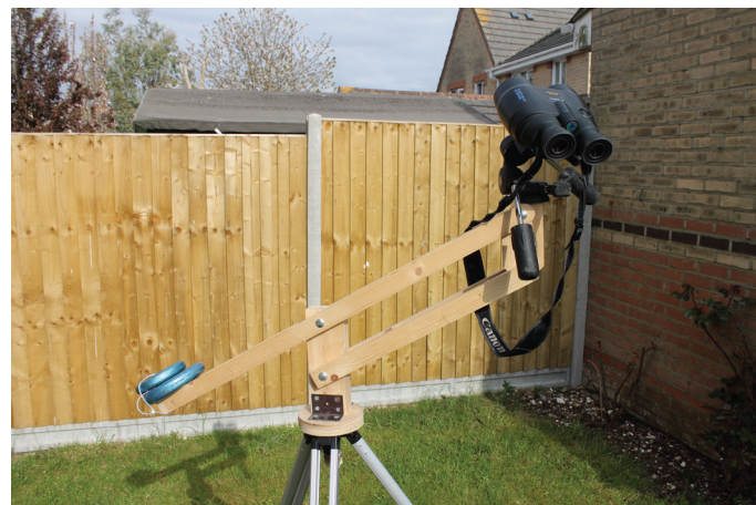
▲ A simple parallelogram mount holding 15 × 50 binoculars providing comfortable viewing at any position. Image: Mark Radice.
