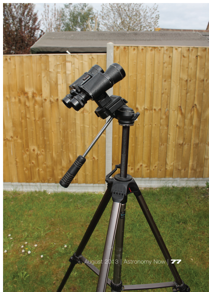
▼ A pair of 7 × 35 binoculars held on a camera tripod. This works perfectly well until 45 degrees elevation where it becomes increasingly hard to get to the eyepieces. Image: Mark Radice.
